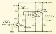
Generator circuit with charge time equal to flyback time.
