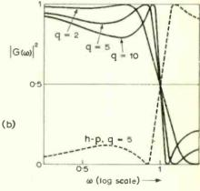
Fig. 4. 3rd-order responses obtainable from active parallel-T system. Note linear power scale.
