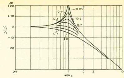
Fig. 10(a).  $\frac{V_2}{V_1} = \frac{p_1 p_2}{(p-p_1)(p-p_2)}$  for various values of 1/2Q<sub>0</sub>
