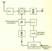
Fig. 5. Phase-locked synthesizer using digital techniques.
