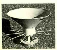
vertex of the cone for structural strength and waterproofing. It is supplied with a base flange for mounting. The frequency range is 250-1000MHz, radiation pattern omnidirectional, input impedance 50Ω, input power 750W, and weight 4kg. Microwave International (U.K.) Ltd., 33-37 Cowleaze Road, Kingston upon Thames, Surrey.
