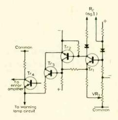
Fig. 4. Simplified current limit circuit.
