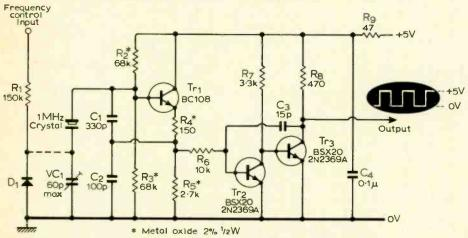
Fig. 7. Complete circuit of the 1MHz oscillator. The final two transistors form a shaping circuit to provide the required square-wave output.
