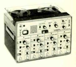
they can be further improved with electronic flutter compensation. Channel 4 has three modes of operation: data only, voice only and data interrupted by voice. A useful built-in feature is a c.r.t. monitor which displays the deviation of all four channels simultaneously and facilitates selection of the appropriate input range. The instrument weighs 11.3kg and measures 330 × 240 × 270mm. Farnell Instruments Ltd, Sandbeck Way, Wetherby, Yorks, LS22 4DH.
