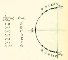
Fig. 10(b). Roots corresponding to responses in 10(a).
