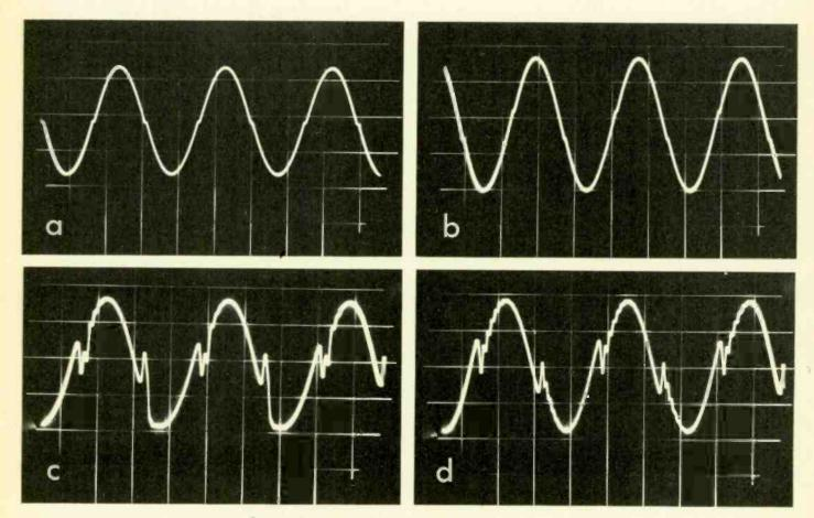
Fig. 1. Crossover distortion in a class B stage employing transistors with an  $f_{\tau}$  of about 2MHz. (a) Low frequency sine wave at 10mA. (b) High frequency sine wave showing the effect of hole storage on the crossover discontinuity under light load conditions. (c) Influence of hole storage and n-p-n/p-n-p asymmetry under high current conditions at 200kHz. (d) Improvement of conditions in (c) by reducing source impedance.
