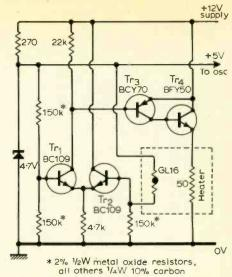
Fig. 1. Initial experimental temperature control circuit for the crystal oven.
