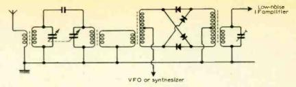
Fig. 7. Even without an r.f. amplifier, diode-ring mixers using Schottky (hot-carrier) diodes can give low-noise performance with wide dynamic range.
