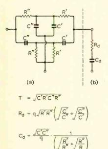
Fig. 9. Balanced parallel-T network constructed from matched pairs of components.
