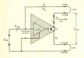
Fig. 1 (left). Voltage control block diagram—voltage calibrator.
