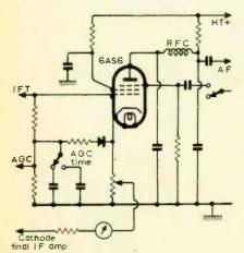
Fig. 11. Philco combined.a.m. /s.s.b. demodulator.
