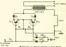
Control circuit with low power dissipation when off.
