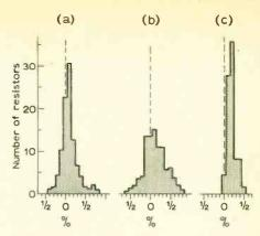
Fig. 3. Typical test results showing the percentage change of resistance for given conditions. (a) Conditions as per DEF5115/RFG5F at rated volts at 70°C for 2000 hours; spec. limit ±3%. (b) Same conditions as (a) but for 10,000 hours. (c) Tropical exposure with light load for 1,344 hrs; spec. limit ±1%.
