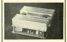
Using the article as published in the January 1970 issue of Wireless World, a universal printed-circuit board has been designed suitable for both positive and negative earth ignition systems. This also enables simple conversion to opposite polarity if the vehicle is subsequently changed.
