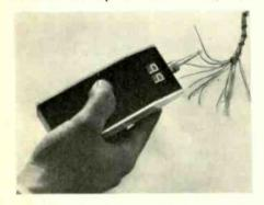
self-powered versions for use inside aircraft or where mains supplies may not be available. The instrument is not affected by cable capacitance, resistance, or inductance, and no damage can be caused to low-power components which are joined to the wires under test. Information Computer Systems Ltd, Mill Street, Crewe, Cheshire.
