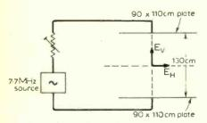
Fig. 3. Diagram of capacitor.
