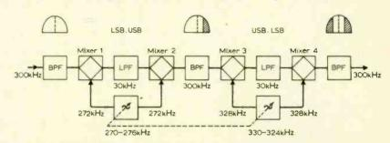
Fig. 8. Rohde & Schwarz variable-bandwidth i.f. filter shown set for  $\pm$  2kHz bandwidth.
