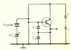
Fig. 6. Basic circuit of the oscillator.
