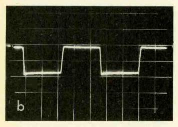
Fig. 5. Amplifier response driving a reactive load (15  $\Omega$ , 0.47  $\mu$ F) with a 10kHz square wave. (a) The ringing gives evidence of instability. (b) No transient ring indicates better stability.
