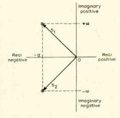
Fig. 1. Frequencies in the complex plane.
