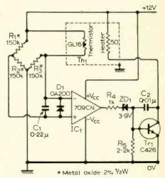
Fig. 2. Temperature control circuit actually used. Improved performance is obtained because of the higher loop gain.
