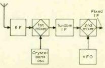
Fig. 2. Multi-conversion superhet having crystal-controlled first oscillator.
