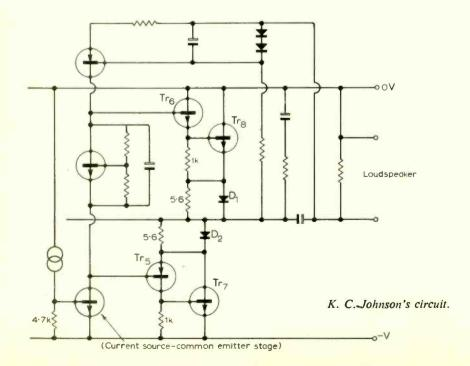
Mr. Baxandall's letter is also the source of another refinement. The diode-dodge, which is the main topic of his letter, may not bring such a pronounced improvement to K. C. Johnson's circuit (due to the different quiescent driver-currents in the different circuits Mr. Johnson's power transistors cut out at much lower signal levels) but it may be worth trying—particularly since the components are so few.
