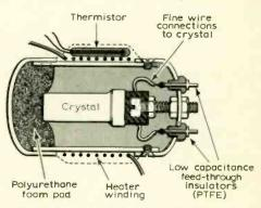
Fig. 3. Cross-sectional diagram of construction of the oven.
