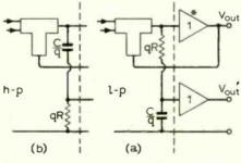
Fig. 2. Use of damping branch to give 3rd-order response.
