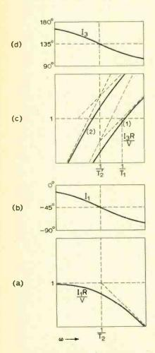
Fig. 6. Phase and amplitude plots of the short-circuit output currents of the two tees for constant input voltage.
