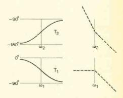
Fig. 14. Phase and asymptotic gain diagrams for the two portions of the loop.
