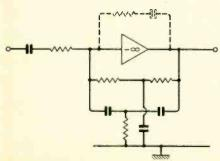
Fig. 11. Parallel-T selective amplifier
