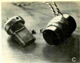
Fig. 4. (a) The oven with the heater winding in place over the insulating paper tape. (b) The heater and thermistor in place, with connecting wires attached. (c) Completed oven, opened to show the crystal in position in its socket.
