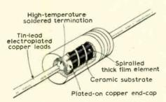
Fig. 1. The construction of a metal glaze resistor.
