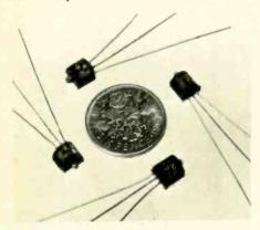
dimensions of 5mm. The circuit contains one transistor, one diode and two resistors and is designed to operate from a 5-V 4-mA supply. It indicates logic states of "O" (0.5V lamp off) and "1" (2.5V lamp on) with input currents of  $5\mu$ A and  $30\mu$ A respectively. Newmarket Transistors Ltd, Exning Road, Newmarket, Suffolk.
