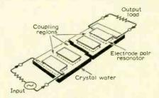
Fig. 1 Monolithic h.f. crystal bandpass filter.
