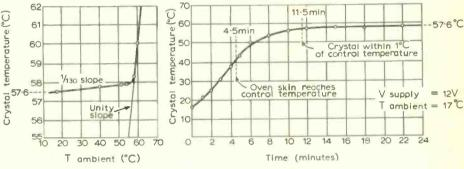
Fig. 5. Warm-up curves for the oven, obtained with a calibrated thermistor.
